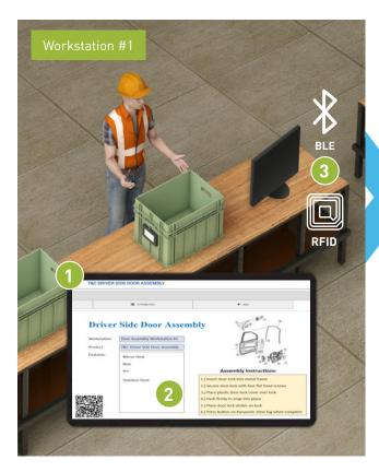
Process Details shown only for that specific workstation and assembly step
